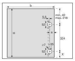
if width **b** increases, measurement **a** must also be increased
